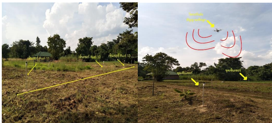
Figure 4 The arranged of soil moisture sensors and the experimental test with drone flying.
