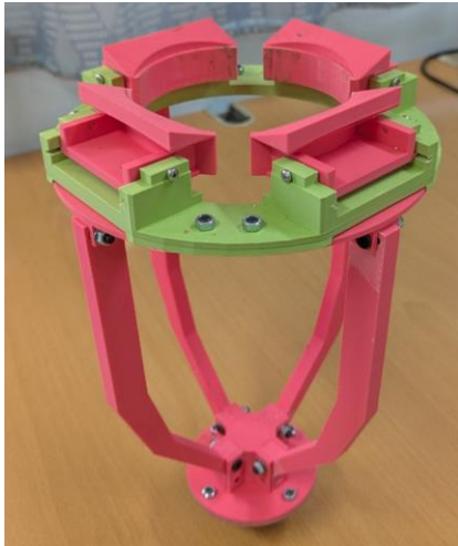
Fig 2. A 3D-printed prototype of the developed adjustable end-effector.
