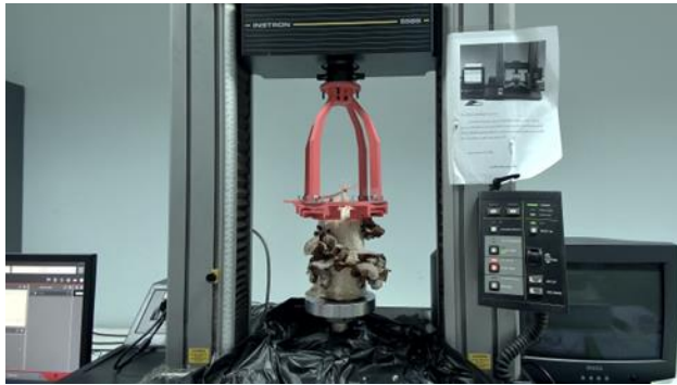
Fig 3. Arrangement of the mushroom bag sample and the end effector with the universal testing machine in mechanical tests.
