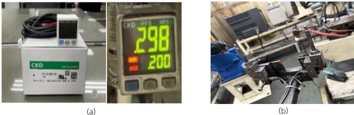
Figure 3 Materials and methods. (a) Digital pressure sensor. (b) Poka-Yoke (Inductive sensor and guide pin).
