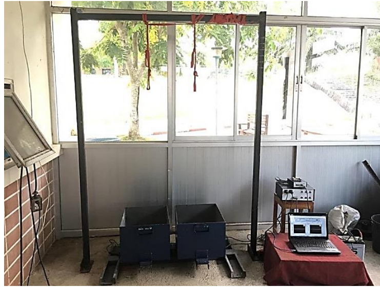
Figure 3 Apparatus for measuring reaction forces during the extraction of boots from wet soil.
