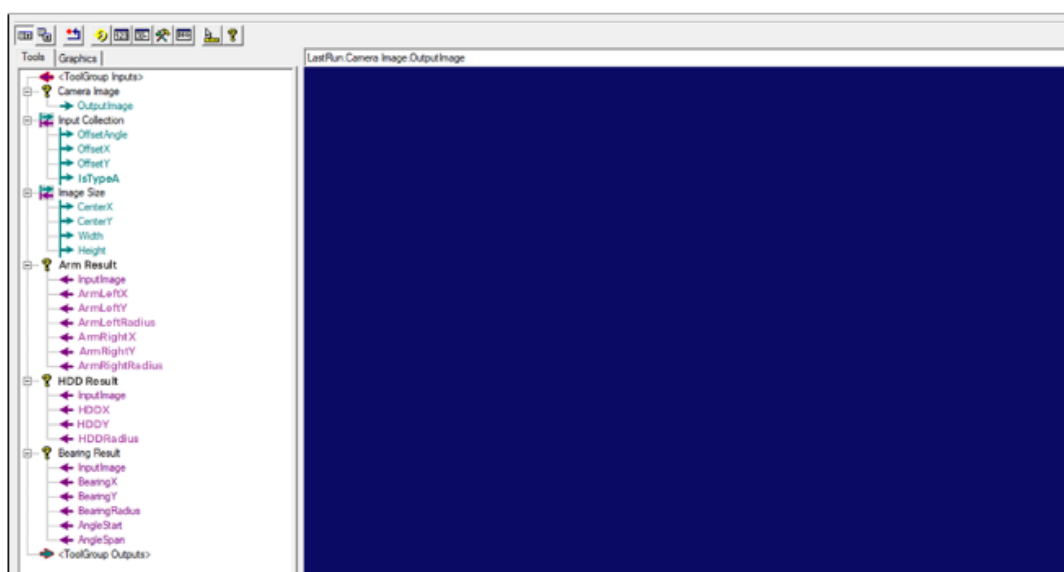
Figure 4 Internal structure of basic tools within the automatically generated Recipe file
