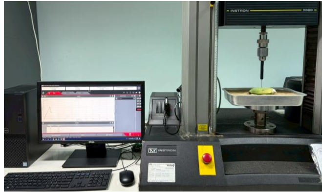
Figure 2 Firmness measurement of Namwa banana using a universal testing machine.
