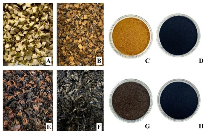
Figure 1 Physical characteristics of durian peel and the activated carbon process. (A-D) Control group: (A) durian peel, (B) Dried durian peel, (C) NBPD Powder, (D) Activated carbon from durian peel, (E-H) Preparation of activated carbon by fungal activation: (E) Durian peel and P. palmivora (F) Biological Pretreatment Durian peel (G) BPD Powder (H) Activated carbon from Biological Pretreatment durian peel.
