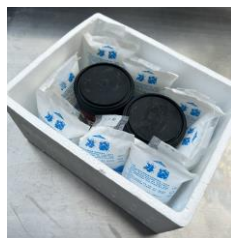
a) Arrangement of two cans of frozen marinated salmon and eight gel ice packs inside a foam box.
