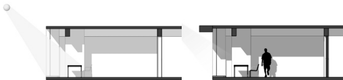
Fig 4: (Left) Light Penetration on March 21 at 8am on existing condition (Right) Light Penetration on March 21 at 8am with static shading
