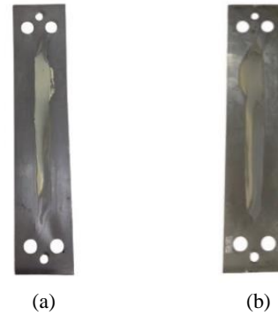
Fig. 4. fouling thickness (a) PID temperature control system (b) ON-OFF temperature control system at 300 seconds.
