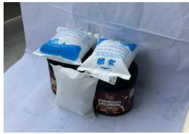
a) Arrangement of two cans of frozen marinated salmon and four gel ice packs before wrapping with heat-reflective aluminum foil.
