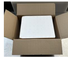
b) Placement of the foam box inside B-flute corrugated mailer.
