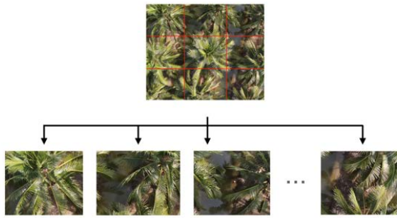
Fig. 4. An example of how to partition an image into 9 sub-images.
