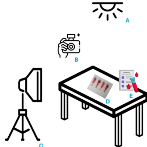
Fig. 2. The configuration of capturing the microfluidic chip: (A) White light color, (B) Camera capture by researcher using a mobile phone with resolution of 3000x4000, (C) Tripod light with 60W 5400K (D) Microfluidic chip, (E) Standard red cells solution according to the Thai Red Cross Society.
