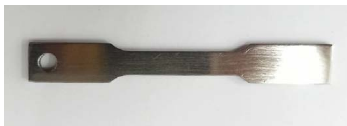
Figure 2 Subsize Specimen according to ASTM E8/E8M – 13a (2).
