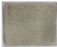
Figure 2 Tile made from clay combined with oil palm ash, spent bleaching earth, and palm fiber.
