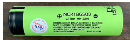
Fig. 1. Panasonic NCR18650B (NCA cylindrical Li-ion batteries).
