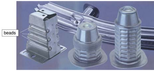
Fig. 2. Crash-boxes used on automotive bumpers. Image: [10]
