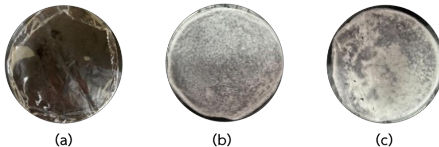
Figure 1 The images of (a) PVA film, (b) PVA-5%CL film and (c) PVA-10%CL film.
