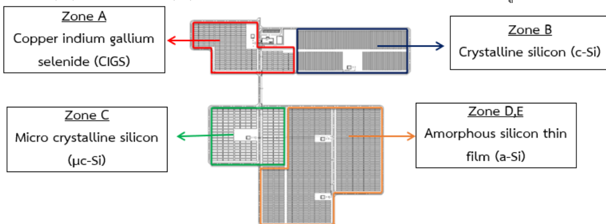
Figure 1 Diagram of PV technologies and photovoltaic systems at Thap Sakae solar farm, Prachuap Khiri Khan.
