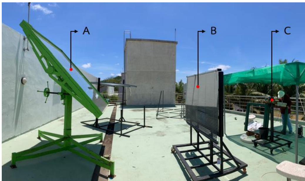
Figure 2 Photograph of the experimental set-up: (A) solar reactor, (B) heliostat and (C) fresnel lens.
