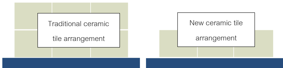
Figure 6 Comparison of ceramic tile placement on pallets original and new.
