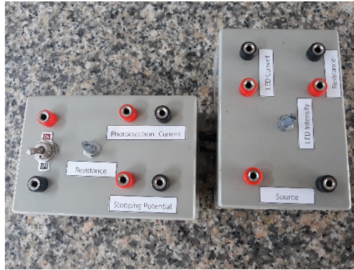
Figure 1 The apparatus used for demonstration of the photoelectric effect.
